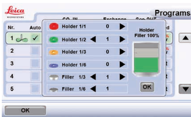
Pop up-filler display: Filler and sample holder settings affect process time. Automated adjustment of the CO 2 IN time, exchange time and gas OUT time to filler-holder status.
