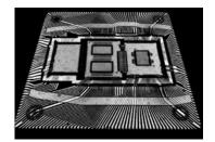
G-Scan (Gate-Scan) produces multiple images depending on the "gate memory". Different settings can be stored for automatic evaluation.
