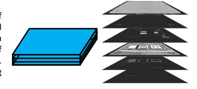
Z-Scan - Automated volume acquisition which enables an offline reconstruction of B-, C-, D-, P-, X-, A-, 3D-Scans and time of flight images with free selectable gate windows
