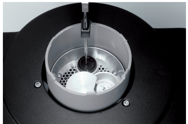
After freezing the grid remains in or above ethane (depending upon user settings), ready for transfer to the grid box.
