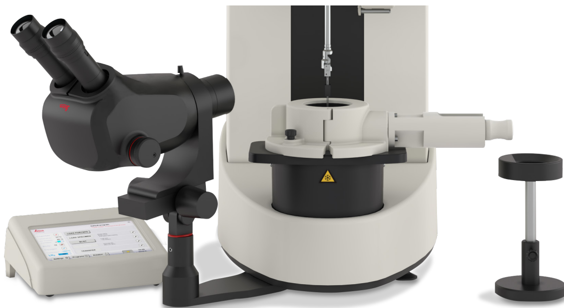
EM GP2 with Cryo-TEM transfer adapter mounted. Additional Cryo-TEM support is visible below the cryo-TEM holder entry.
